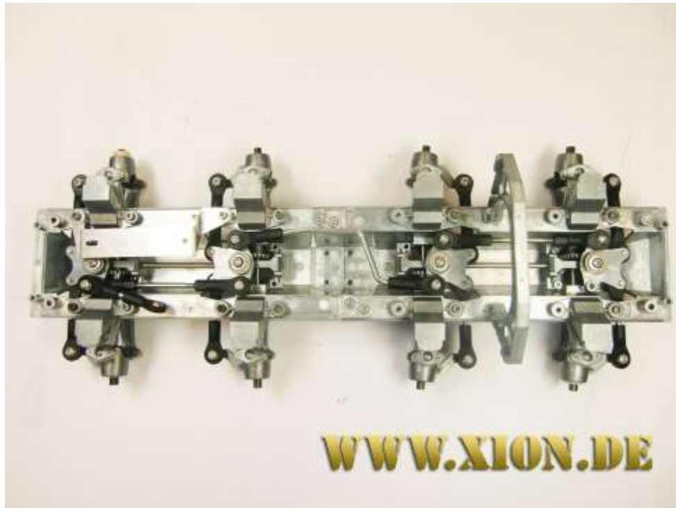
Alternate assembly of steering linkage
